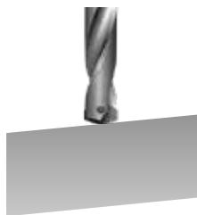
The approach angle between Drill and the workpiece at the beginning and the end should be less than 6°. Reduce the feed (fn) to 30-50% than general cutting conditions at the beginning and the end of angled surface.
