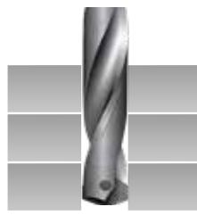
Gap between the plates could make wrong chip evacuation causing fracture of the Drill. Place stacked plates without any gap between each.
