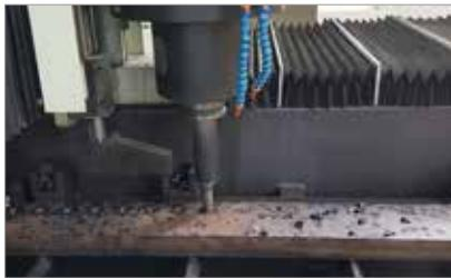
**Cutting condition**  $vc = 60 \text{ m/min} \cdot fn = 0.25 \text{ mm/rev} \cdot ap 50 \text{ mm} \cdot \text{Nass}$
