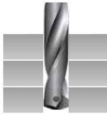
Gap between the plates could make wrong chip evacuation causing fracture of the Drill.
