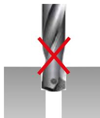
Boring is not recommended due to wear and chipping in the corner of the insert.
