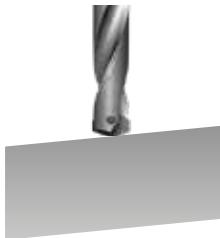
The approach angle between Drill and the workpiece at the beginning and the end should be less than 6°.
