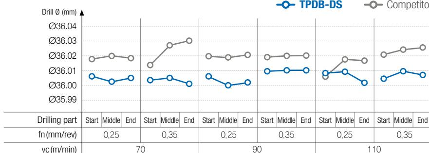
» Improved machining precision through double margin and stable chip evacuation.
