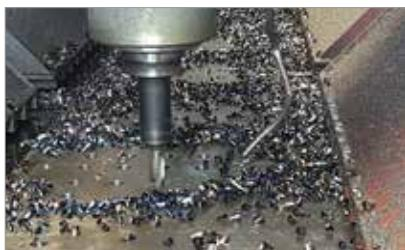
**Cutting condition**  $vc = 70 \text{ m/min} \cdot fn = 0.25 \text{ mm/rev} \cdot ap 24 \text{ mm} \cdot \text{Nass}$
